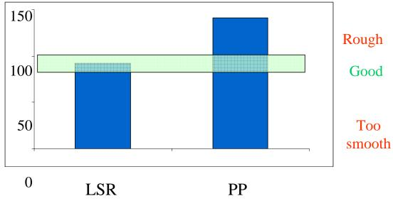
In the graph the Leroux tests done by Labosport France are shown. The Leroux value gives an indication of the field, whether it is good, too rough or too smooth. It is clearly shown that LSR® is positioned in the safe area.
