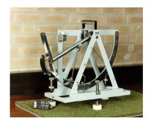
The underfoot friction is important for the players in order to reduce the risk of foot blocking during the foot-surface interaction. The method is different from the traction test, but it is measuring the same subject. Underfoot friction is obviously a measurement of the slipperiness of the surface and is measured using the Leroux machine as modified by NOC\*NSF (Dutch Sports Federation).
