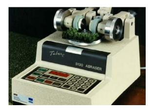
Fibres used in the sports surface industry must resist player and climate influences. One of the test methods available is the Taber test. In this test, two small, roughened wheels carry out a combined rolling/sliding movement across an artificial grass sample, indicating the wear resistance of the surface. This test can be done with both new and aged material, but is only useful for testing samples of water based pitches.
